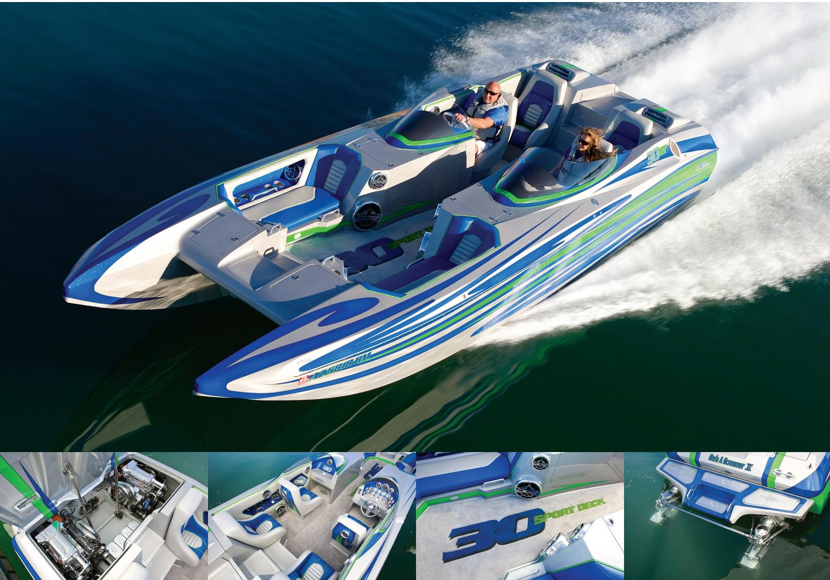
From left: Dave's Custom Boats did a fine job when it came to rigging the twin 900-horsepower engines. The cockpit featured four high-back bucket seats. Custom touches included the 30 Sport Deck name in the carpet as well as speaker covers with the DCB logo. The boatbuilder designed a new two-tier swim platform for its first deck boat.
