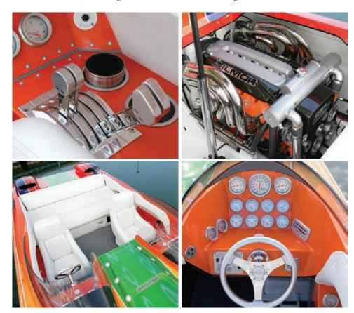
Clockwise from top left: Latham Marine throttles and shifters were right of the driver's seat. Ilmor's 625-hp V-10s powered the boat to better than 120 mph. The helm looked more like an airplane cockpit than that of a performance boat. The rear four-person bench was uncommonly deep and the buckets were comfortable.
