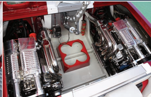
From left: The starboard-side driver's station resembled a jet with its quarter-canopies and rows of Livorsi Marine gauges in chrome bezels. Between each of the bucket seats in the rear was a cupholder, a billet step plate and a grab handle. Two supercharged 1,100-hp engines from Teague Custom Marine supplied power to the catamaran.
