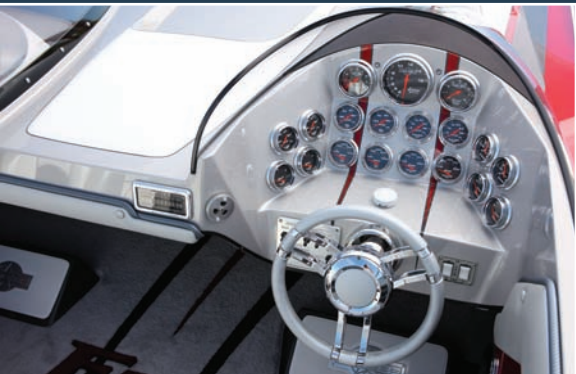
From left: The starboard-side driver's station resembled a jet with its quarter-canopies and rows of Livorsi Marine gauges in chrome bezels. Between each of the bucket seats in the rear was a cupholder, a billet step plate and a grab handle. Two supercharged 1,100-hp engines from Teague Custom Marine supplied power to the catamaran.
